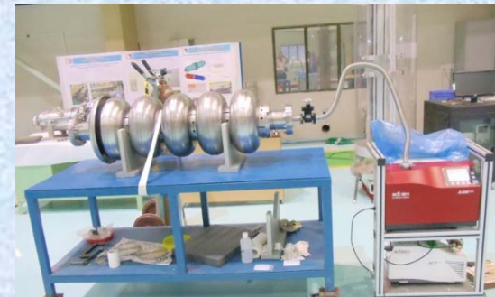
“Vacuum leak testing Leak rate < 10^{-10} mbar-litres/s
