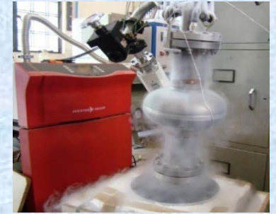
Vacuum leak testing
