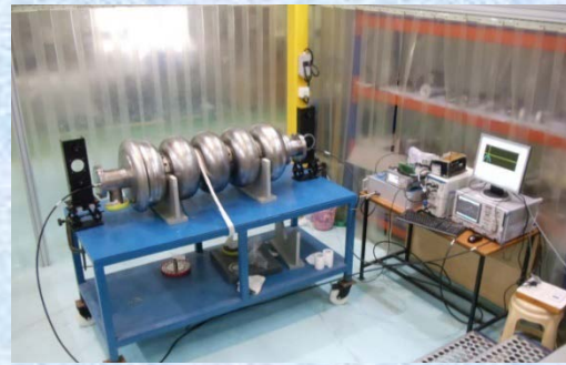
“RF qualification Frequency at 300 K: 649.5922 MHz Field Flatness ( as fabricated) = 68%.
