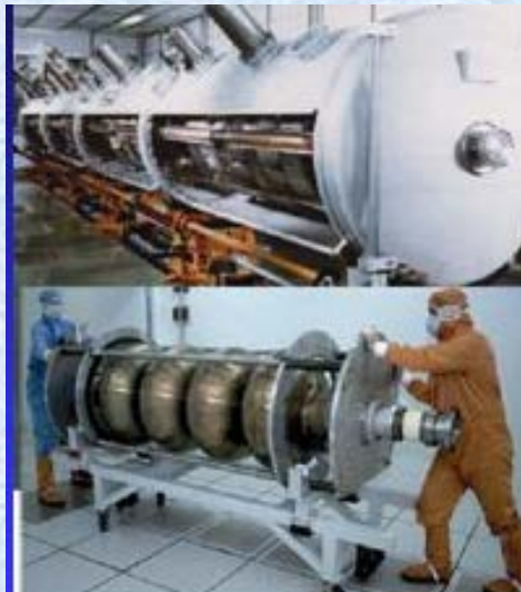
LEP NB coated Cu cavities 15 MV/m @400 MHz
