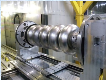
“1 st Five-cell SCRF cavity RRCAT-HB92-5001”. Total length 1403 mm
